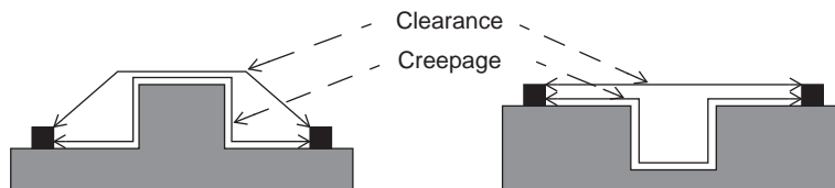
FIGURE 39.2: Creepage and clearance distance
