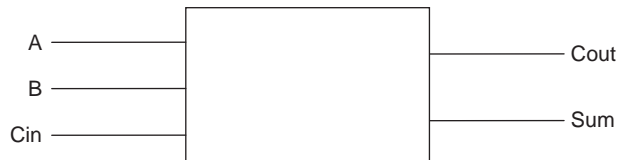
FIGURE 10.9: One-bit full-adder cell
