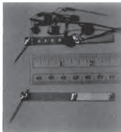
FIGURE 1.157: This probe circuit's input impedance is 10^{11} \Omega in parallel with 0.29 pF (A). Optimized primarily for its impedance characteristics and not its frequency response, the probe's bandwidth and slew rate are 90 MHz and 300V/ \mu s, respectively. If the lack of physical rigidity of the TO-92 packaged FET makes it too wobbly to use as a probe, a piece of 1/16-in. glass epoxy board with the copper peeled off will add rigidity with only 0.08 pF of additional capacitance. The layout of the drilled-out beam shown in the top of Figure 1.157(B) adds only 0.06 pF to the input capacitance.
