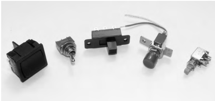
FIGURE 1.19: Various types of switches. From left to right: a mains rocker switch, an SPDT miniature toggle (changeover) switch, a DPDT side switch, an SPDT push-button (wired for use as an SPST push-button), a miniature PCB mounting DPDT push-button (with a latching action).
