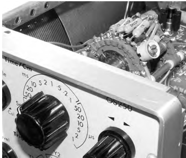
FIGURE 1.94: C-R circuits are widely used in electronics. In this oscilloscope, for example, a rotary switch is used to select different C-R combinations in order to provide the various timebase ranges (adjustable from 500 ms/cm to 1 \mu\text{s/cm} ).
