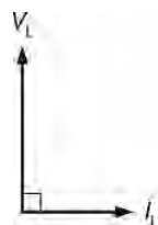
FIGURE 1.114: Phasor diagram for a pure inductor
