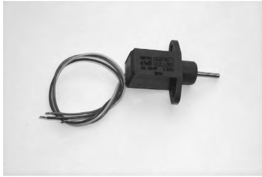
FIGURE 21.5: Resistive linear position sensor
