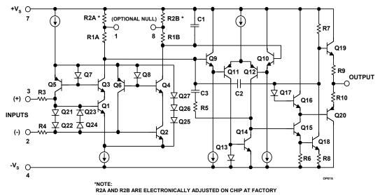
Figure H-22: The OP07 monolithic IC op amp
