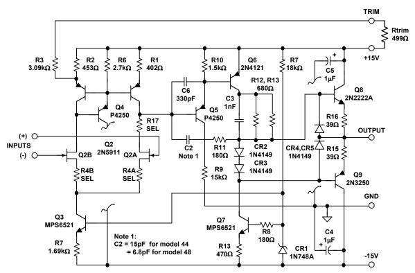
Figure H-12: The ADI model 44 and 48 high speed FET-input modular op amps
