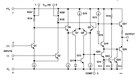
Figure H-21: The µA725 monolithic IC op amp
