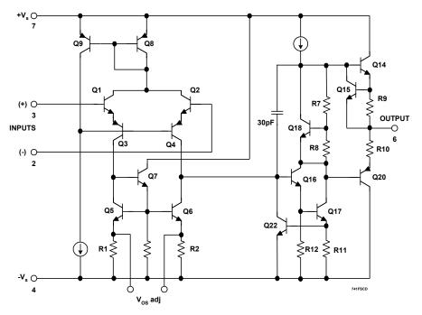
Figure H-17: The µA741 monolithic IC op amp
