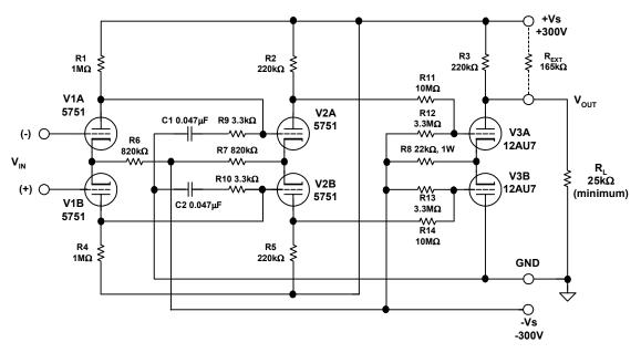
*Figure H-6:* A fully differential op amp design by Bela Losmandy, for Micro-Gee Products, Inc.
