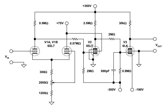
*Figure H-4:* Schematic diagram of late M9 system op amp designed at Bell Telephone Laboratories
