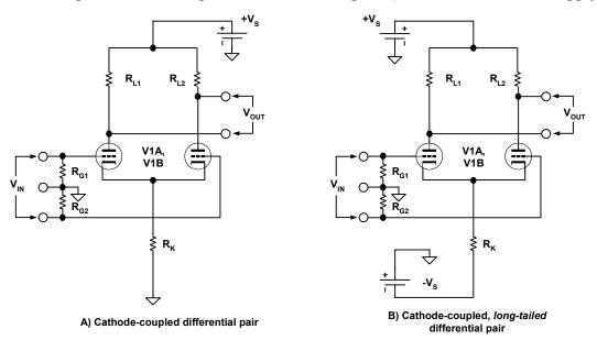
**Figure H-2:** A comparison of simple differential pair biasing in A (left) and longtailed biasing as in B (right)
