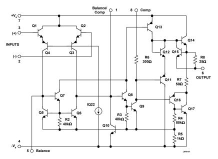
Figure H-16: The LM101 monolithic IC op amp
